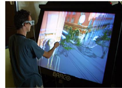
Semi-immersive VR using the Barco Baron workbench (Drettakis, Roussou, Tsingos, Reche & Gallo, 2004).
