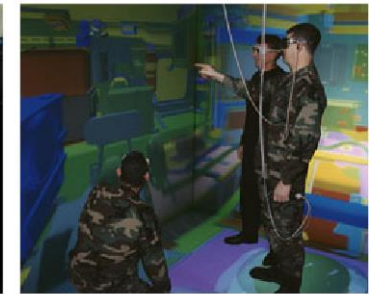
Projection-based immersive VR. The users are fully immersed in the 'CAVE' (FakeSpace, 2006; Cruz-Neira, Sandin & DeFanti, 1993).
