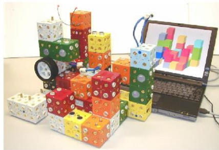
Using physical objects to create a virtual model (Ichida, Itoh, & Kitamura, 2004). As a user adds a physical 'ActiveCube' to the construction, the equivalent virtual model is automatically updated.
